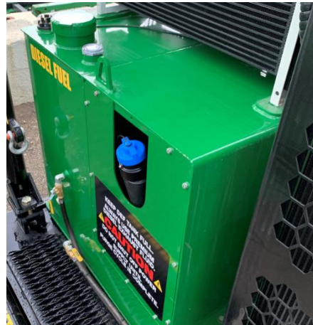
DEF Tank- Storage for diesel exhaust fluid.
