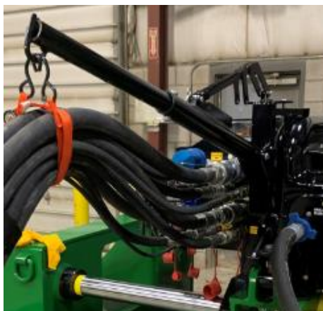
Hose Support- Adjustable bracket that supports all the hydraulic supply umbilical.
