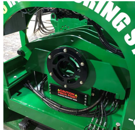
Guide Bearing- Breakout guide bearing can be adapted to any tool joint diameter.
