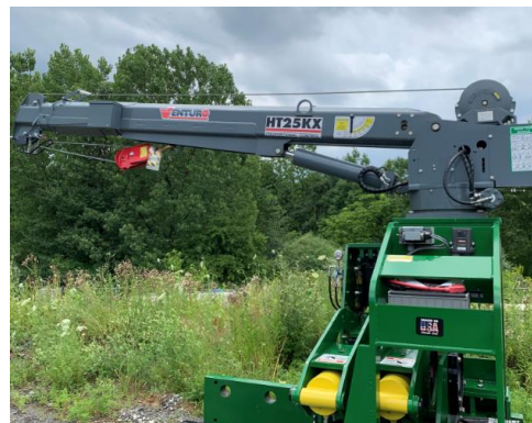
Crane- Full function crane with wireless remote control
