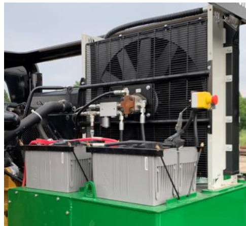
Battery Station- Contains all batteries and main battery disconnect.
