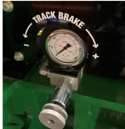
Friction break adjustment- Controls the pressure the friction break delivers.
