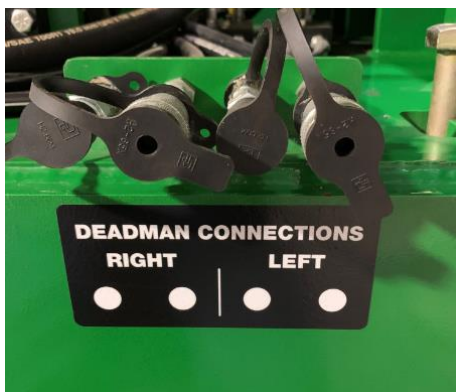
Deadman connections- Hydraulic disconnects located on the front of the breakout.
