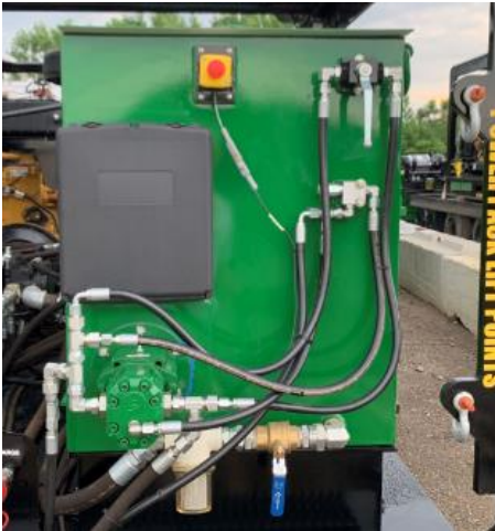
Mixing Station- Control of the mixer prop speed. Containing the fluid pump in-line strainer.
