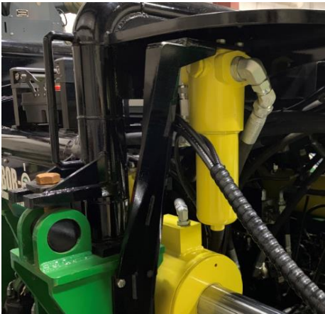
High Pressure Filter- in line open loop filter. Located on the drill unit.
