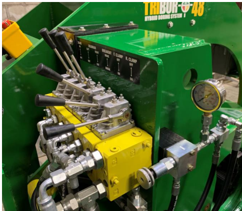
Breakout Control Valve- Controls all the breakout functions.
