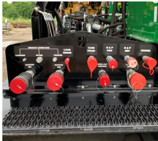
Quick Disconnects- Hydraulic connections to quickly connect all umbilical lines.
