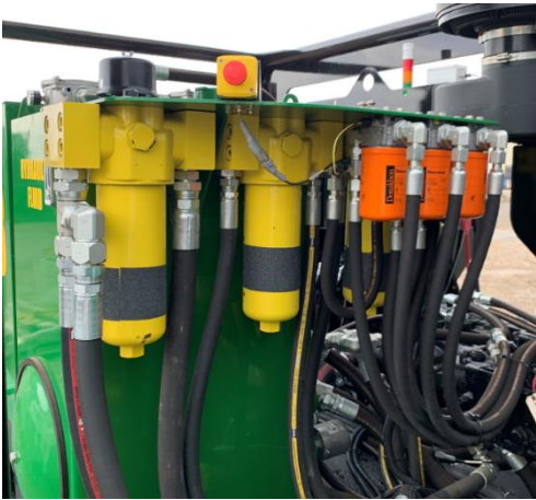
Filter Station- Containing high pressure, and charge pressure hydraulic filters.
