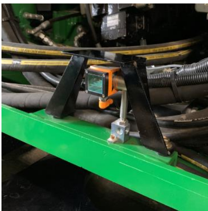
Laser- watches the push bar movement for the auto run function.
