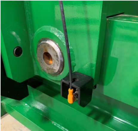
Push Bar Sensor- Locates the dog hole when the push bar is lined up.
