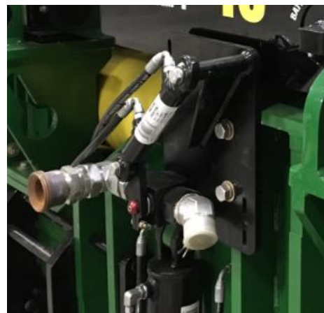
Dump Valve- Hydraulic controlled ball valve designed to dump off excessive pressure in the drill string.
